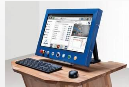
The monitor can be removed for safe operation outside the laser safety barriers.
